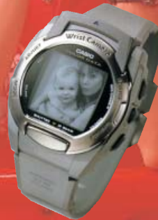
This WRIST CAMERA, our second model, can show images it took in color on PCs, and can hold up to 80 pictures.
