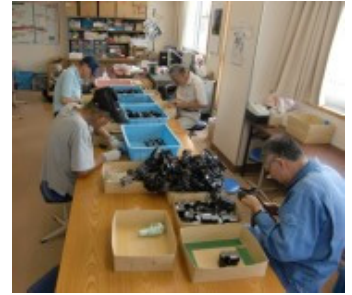
Disassembly and separation of tape cartridges and ink ribbon cassettes
