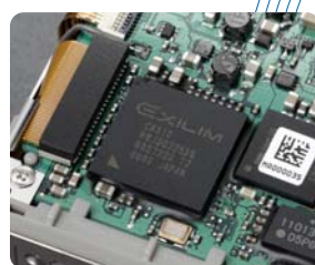
The EXILIM engine, a high-performance image processing module
