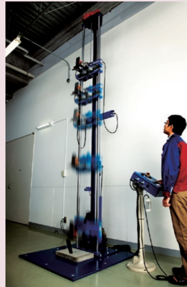
A custom-made drop tester at Casio (350 cm automatic lifting type)
