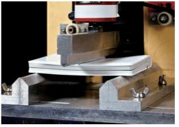
Pressure testing on an electronic dictionary Applying load to the center of the product body, resistance to load from the top is checked
